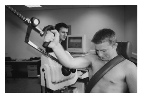
Figure 6.4 Isokinetic dynanometer to measure muscle strength.
