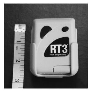
Figure 6.5 Accelerometer.
